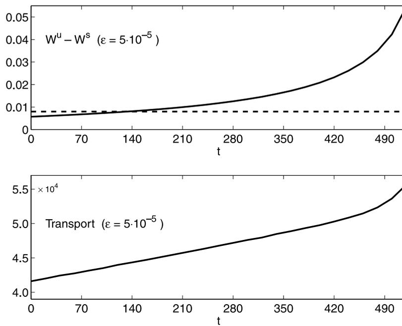
**Figure 6.** Distance between  $W_1^u$  and  $W_2^s$  and the calculated transport for  $\epsilon = 5 \times 10^{-5}$ . The theoretical value of the distance is plotted as a broken line.
