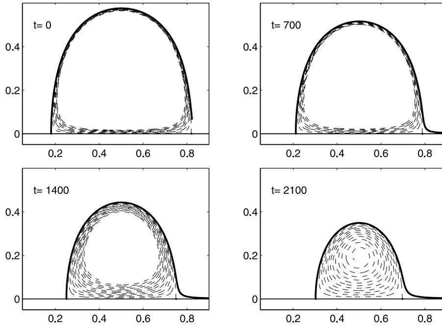
**Figure 2.** Unstable and stable manifolds,  $W_1^u$  and  $W_2^s$ , as computed for the exact solution to the barotropic potential vorticity equation in (5.1) with  $\varepsilon = 1 \times 10^{-5}$ , at times  $t = 0, 700, 1400, 2100$ . The full outer curve is  $W_1^u$  and the broken curve is  $W_2^s$ .
